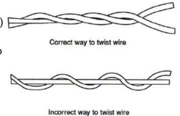
When fitting a capacitor, it needs to be as CLOSE to the motor as possible (even ON the motor is OK!) Always twist the motor and battery wires as shown in the image (**right**). NEVER run the wires parallel to each other like figure-8 cable!
