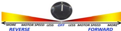
**BOTH DIRECTIONS ON ONE CONTROL METHOD Push Button Braking (SW1 or SW2)
